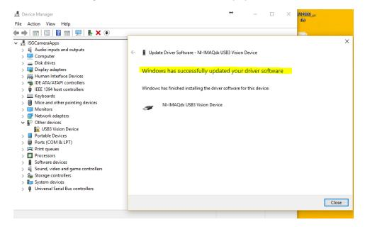
In the device manager, the camera should now show as a NI-IMAQdx USB3 Vision Device.
